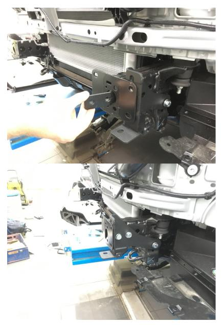
15. Install the frame booster (pos. 4). To do it, screw in the bolt M12x25x1.25 (pos. 19) with washer (pos. 31) in the factory hole; insert the insert sleeve (pos. 10) into the frame; fasten with bolts M12x30 (pos. 20) and washer (pos. 31).
