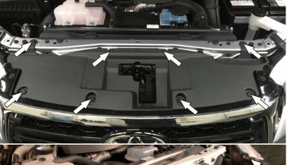
1. Open the hood and remove the plastic patch piece. To do it, remove pop rivets. Keep the fasteners for future mountings.
