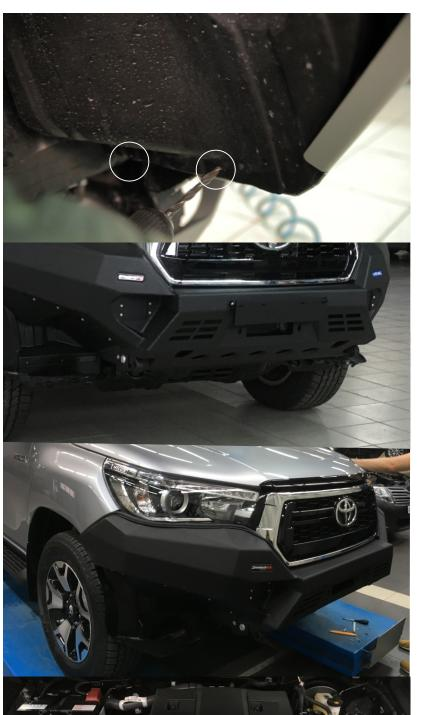
29. From the inner side of the arch, mark two holes in plastic wing flaps opposite to holes in aprons. Drill hole dia. 6 – 8 mm. Through the obtained holes, fasten aprons with screws M6x20 (pos. 22) with penny washers (pos. 28).
