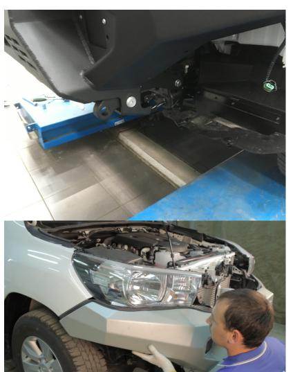
21. Insert screws M10x30 (pos. 23) with countersunk washers (pos. 15) in specified places on the left and right. Fasten to insert sleeves M10 (pos. 11).
