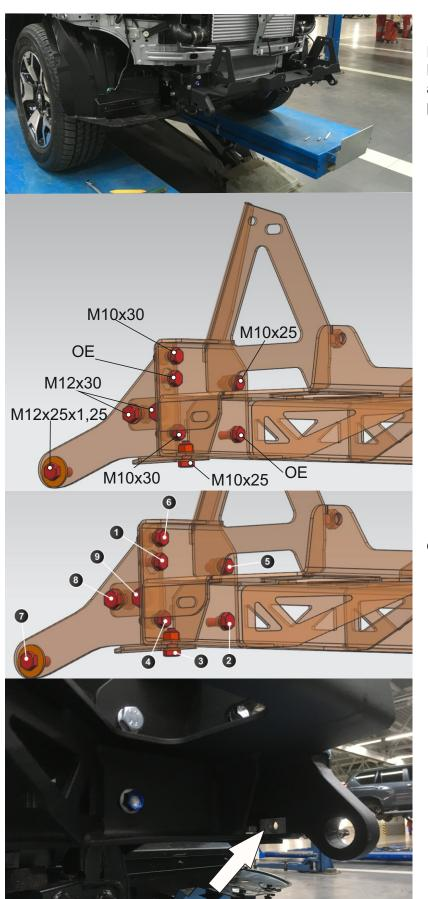
16. Install the winch bracket (pos. 2). Fasten with bolts M10x30 (pos. 18), M10x25 (pos. 17), washers (pos. 29) and nuts 10 (pos. 26). Align the winch pad in vertical and horizontal planes.
