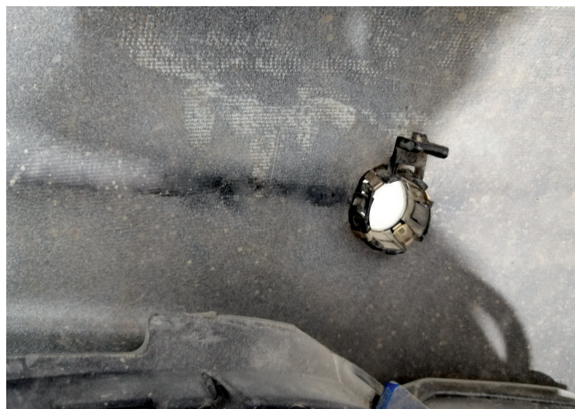
26. Remove parking sensors from factory bumper.
