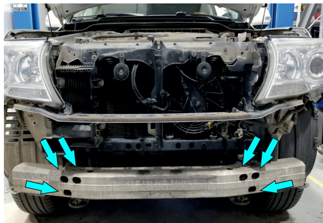
16. Remove damper. Unscrew 3 screws on each side and remove beam.
