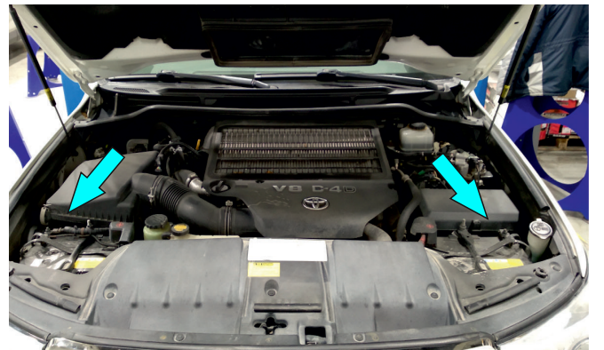
48. Connect all the wires and check it. Install plastic pad in reverse order. Connect terminal "-" of the battery.
