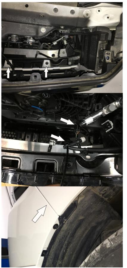
11. Remove all clips, holding bumper with body, under the grill.
