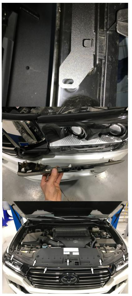
30. Mount radiator grill and fix it using OE fittings in the upper part and screws M6x20 (B) in the lower part.
