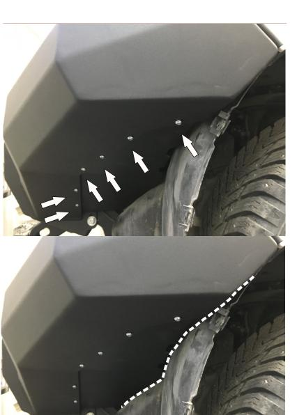
25. Instal caged nuts (D) onto the flaps (5, 6).
