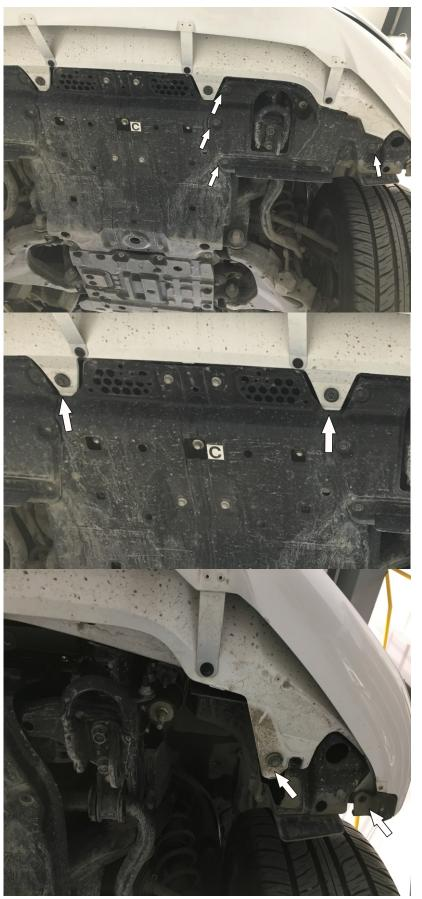
8. Remove lower bumper retaining screws.
