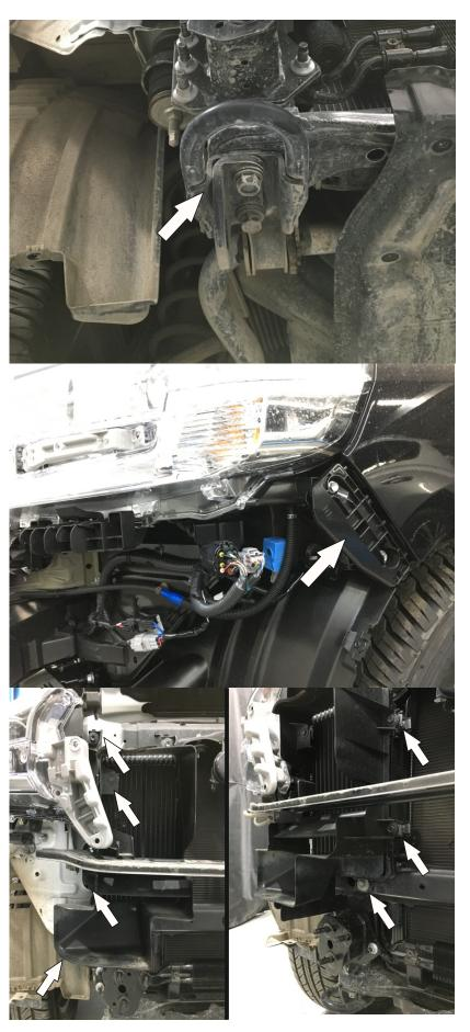
17. Unscrew 2 bolts and remove towing eye on each side.
